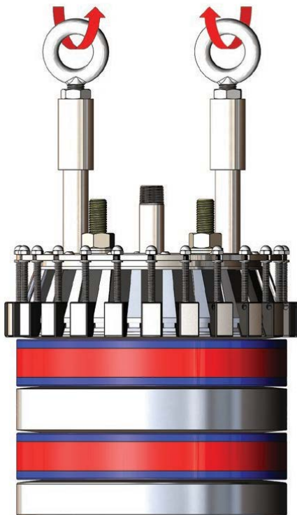
Figure 18: Properly Installed Lifting Eyes for Vertical Lifting
