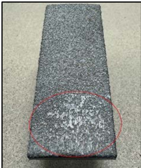
Figure 29: Clogged GritLock Surface
