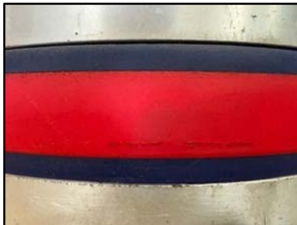
Figure 38: Cracking of Tri-Ply Seal
