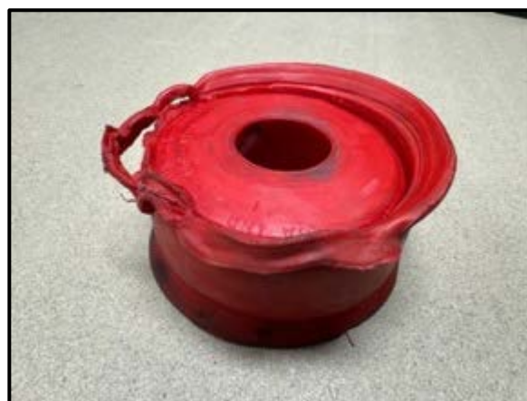
Figure 41: Excessive Deformation of Tri-Ply Seal
