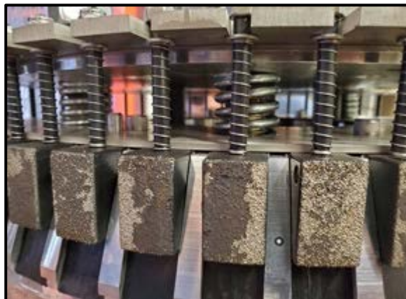
Figure 34: Fouling And Debris On GritLock Surface
