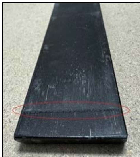
Figure 35: Dented Back Plate
