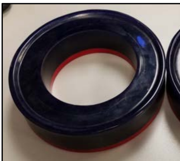
Figure 40: Excessive Deformation of Tri-Ply Seal
