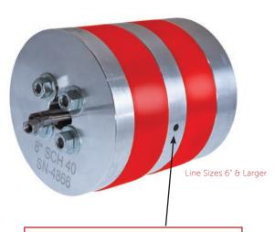
The DBB plug has a vent between the seals that enables you to verify the seal's integrity and pressure test (hydrotest) the welds by positioning the two seals over the weld area.
