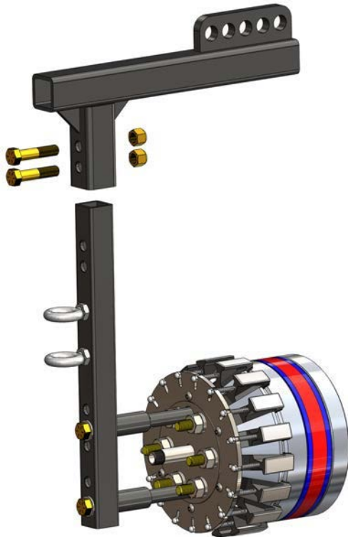
Figure 23: Aligning and Fastening Telescoping Lifting Attachment onto Universal Lifting Bar
