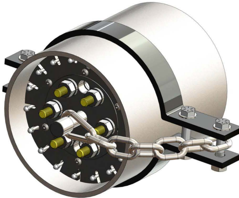
Figure 26: Properly Installed Safety Gag on Pipe
