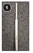
Slide Compression Tube over Extension Rod so that Extension Rod Extends Beyond Compression Tube.
