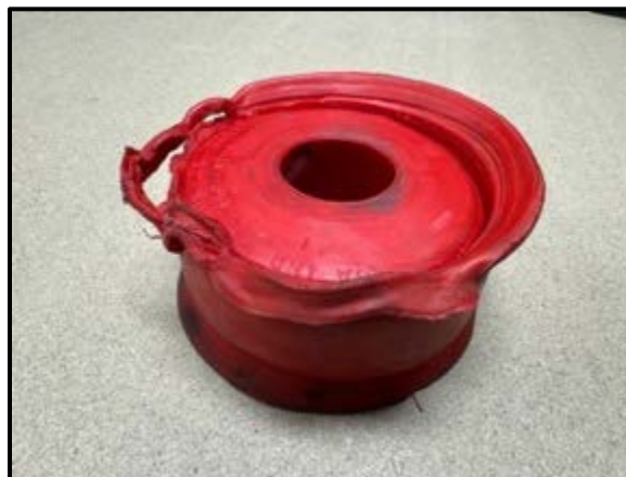
Figure 41: Excessive Deformation of Tri-Ply Seal
