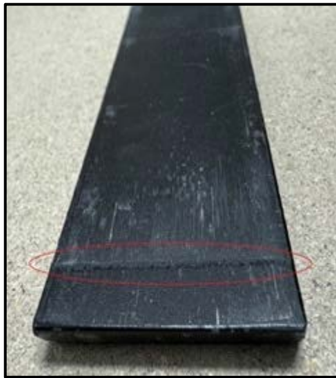
Figure 35: Dented Back Plate
