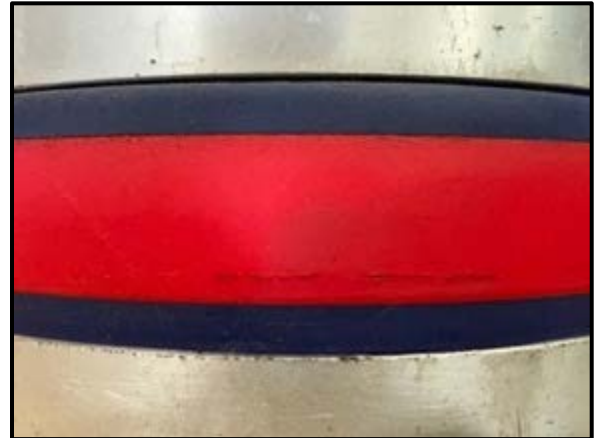
Figure 38: Cracking of Tri-Ply Seal
