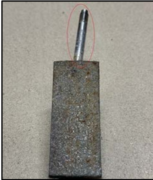
Figure 33: Bent Wedge Stem Circled in Red
