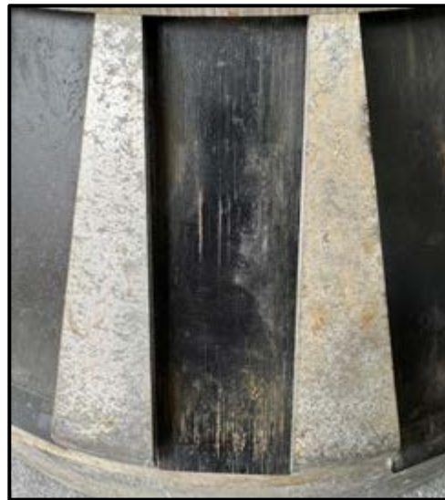
Figure 36: Worn Out And Dirty Back Plate
