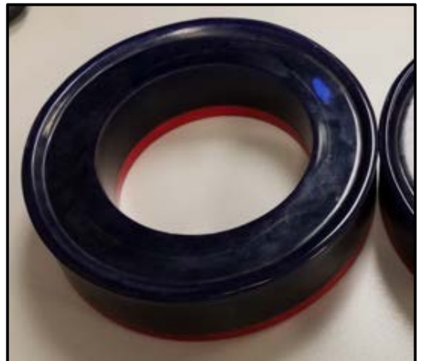
Figure 40: Excessive Deformation of Tri-Ply Seal
