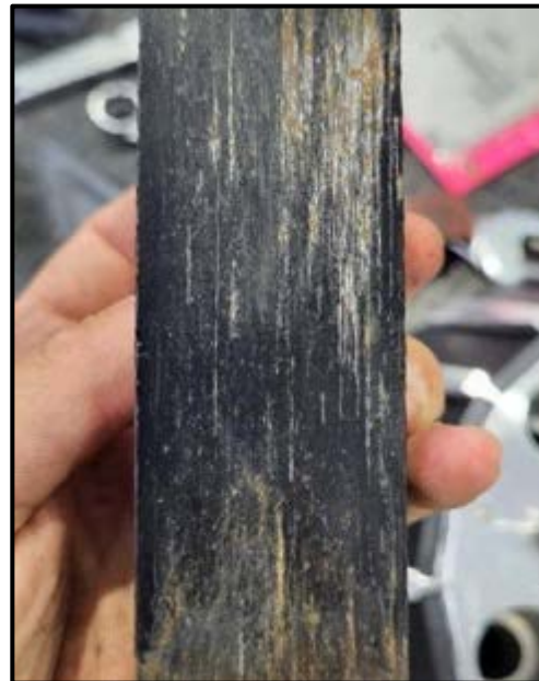
Figure 32: Excessive Wear Of Low-Friction Coating On The Back Side Of Wedge Gripper
