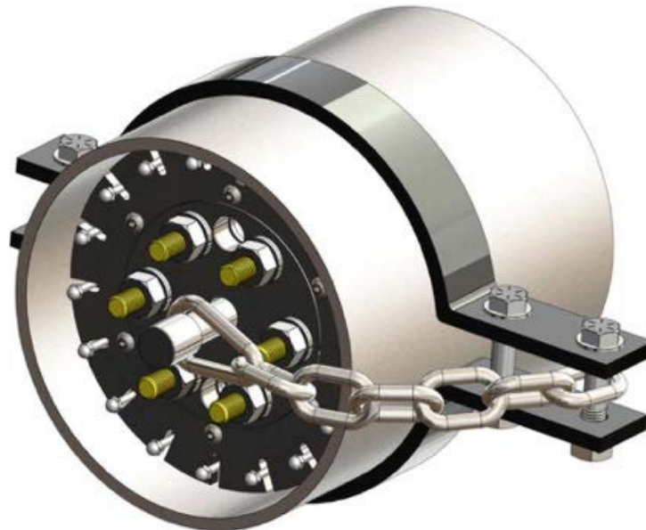
Figure 26: Properly Installed Safety Gag on Pipe
