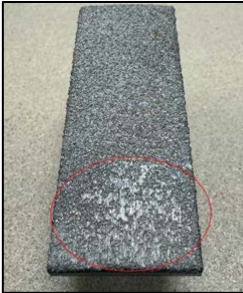
Figure 29: Clogged GritLock Surface
