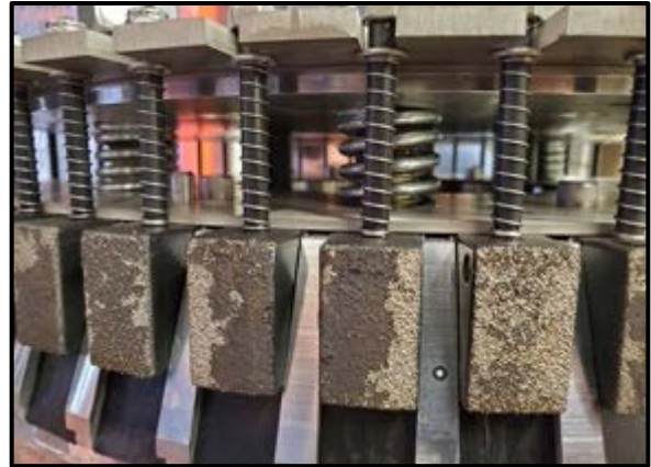
Figure 34: Fouling And Debris On GritLock Surface
