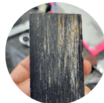
Figure 5: Excessive Wear of Low-Friction Coating
