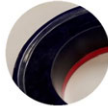
Figure 12: Excessive Deformation of Tri-Ply Seal
