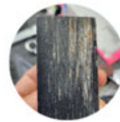
Figure 5: Excessive Wear of Low-Friction Coating
