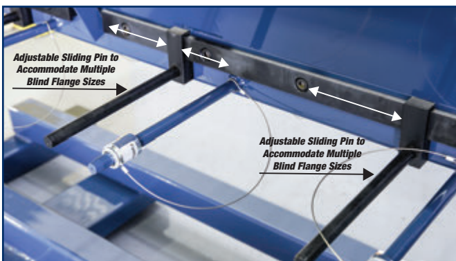
Adjustable Sliding Pins to Accomodate Multiple Blind Flange Sizes
