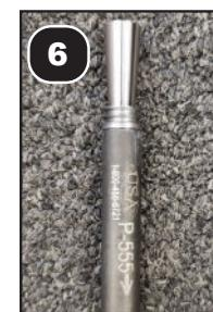
Slide Compression Tube over Extension Rod so that Extension Rod Extends Beyond Compression Tube.
