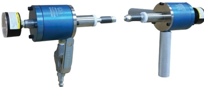
You can leak test rolled or welded tube sheet joints with vacuum pressure in just seconds with the **JLD 2500 Joint Leak Detector**. Insert the nozzle into the tube and press face of the gun into the clean tube sheet joint being tested. Actuate gun to generate the vacuum, if pressure fails to hold...there is a leak.
