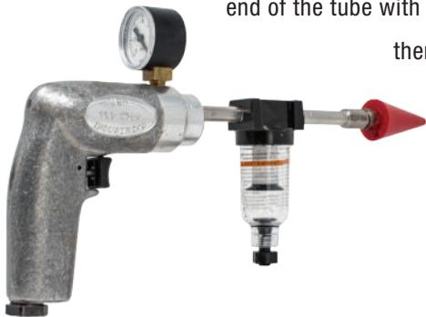
With the **VLD-2500 Vacuum Leak Detector**, simply seal one end of the tube with a rubber plug or a t-handle with a nozzle, then insert the detector into the tube to be tested and press the trigger. If there's a leak, the VLD-2500 reliably detects it with high precision.
