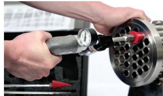
Insert the **TLD 2500 Tube Leak Detector** guns into the tube to be tested. Actuate pressurizing gun by depressing the trigger, the plugging gun seals automatically when pressurizing. After supply pressure is reached, or 100 PSIG (whichever is less), release trigger. If the pressure holds, the tube is OK; if it drops, the tube is leaking - Simple.
